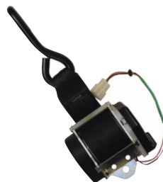
Electric Belt H with hook Length: 3.6 m (front attachment)
