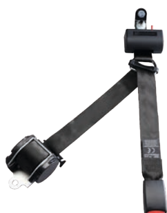
Automatic Shoulder Belt height adjustment with retractor
